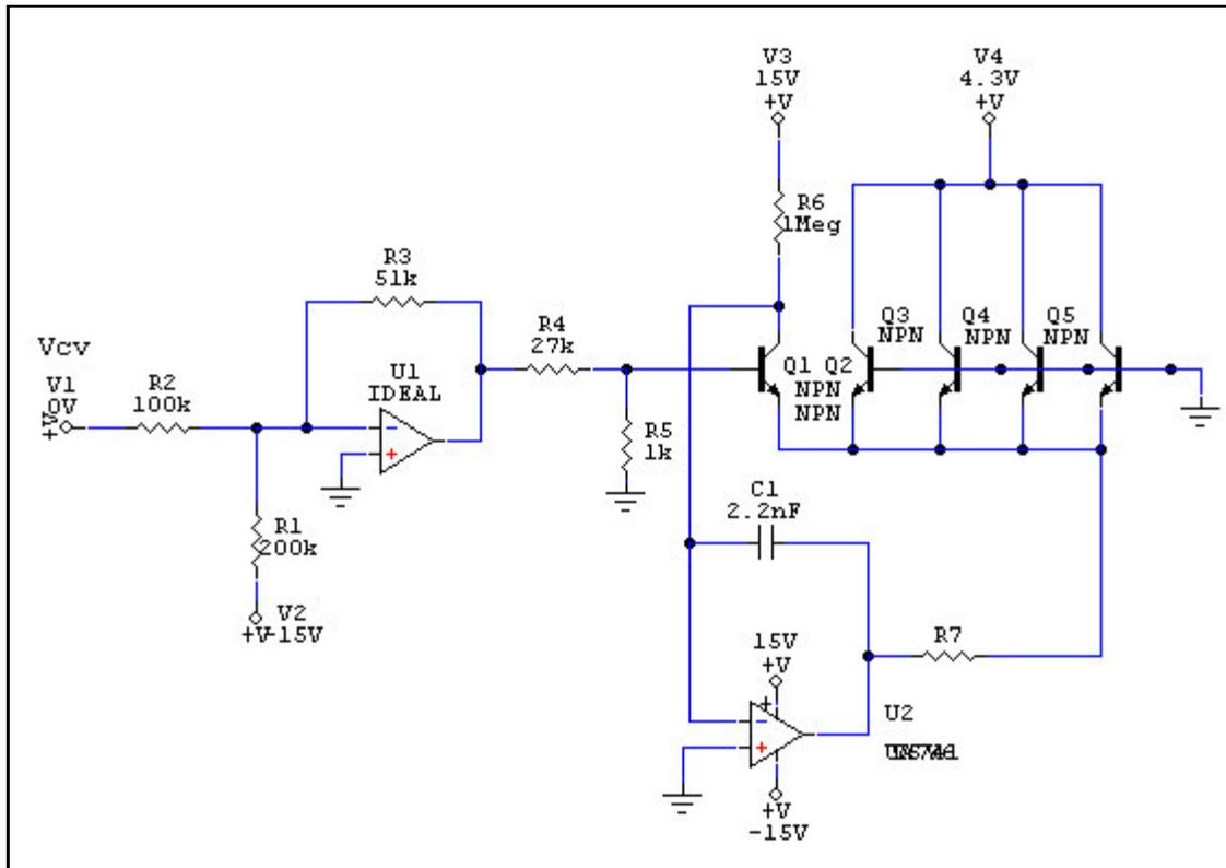
The above circuit is the current sink that generates  $I_{bc}$  for each of the OTAs. The 4 NPN collectors (Q2,3,4,5) are  $I_{bc1}$ , 2, 3, and 4. The resistor R7 (not given a value yet) is used to limit the maximum current of the current sinks (more on this later). First we find the output voltage of the opamp (U1) as a function of the  $V_{cv}$  control voltage:
