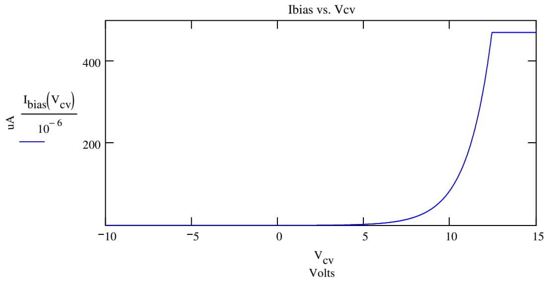
Yes, I did cheat and manually clip the plot at 470 $\mu A$ . One other point to note is that a normal 0..+5V control voltage cannot sweep the filter across it's entire audio range. If this is wanted, then a smaller input resistor on the U1 opamp would achieve this. Perhaps for the second CV input. The first would be labeled 1V/oct and the second could be labeled CV1.
